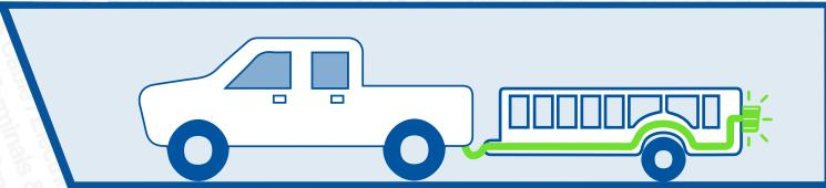
Zip cord is commonly used to wire trailers of all kinds. Many boaters rely on zip cord for their boat trailer wiring needs. The most advantageous aspect is the fact that the parallel bonded conductors are designed to pull apart easily. This means that you can wire one side of the connection and then, as you wire the other side of the connection, you can separate the wires to send each to a separate, specific location.
