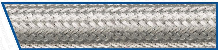
Flat braided cable is a tight weave of soft drawn tinned copper wire. Originally constructed as a tube that is rolled flat creating a specific width. Excellent for use in shielding wire bundle short runs and is easily terminated. Also, flat braid is ideal for use as a low impedance ground path. The flexibility gained from the woven construction and the tinned copper conductors gives this material superb durability against harsh marine conditions.
