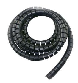
Spiral wrap provides abrasion protection for wire and cable insulation as well as hydraulic and pneumatic tubing. Spiral wrap is also handy for kink-proofing all types of tubing. The spiral cut allows for expandability, easy wire breakouts at any point and excellent flexibility. For maximum abrasion resistance, butt the edges together while installing; for flexibility leave a gap between the edges.
